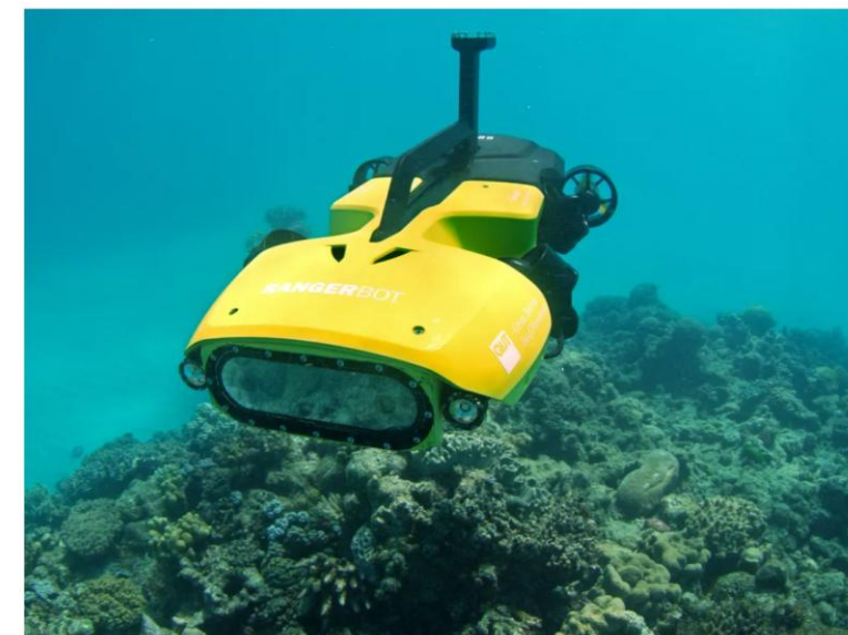
RangerBot is an autonomous underwater vehicle designed to identify and kill crown-of-thorns starfish by lethal injection. Photo courtesy of Queensland University of Technology
